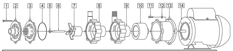
NOTE: When attaching the Drive Magnet to the motor shaft, position the face of the Drive Magnet 3/32 inch below the face of the Motor Bracket
